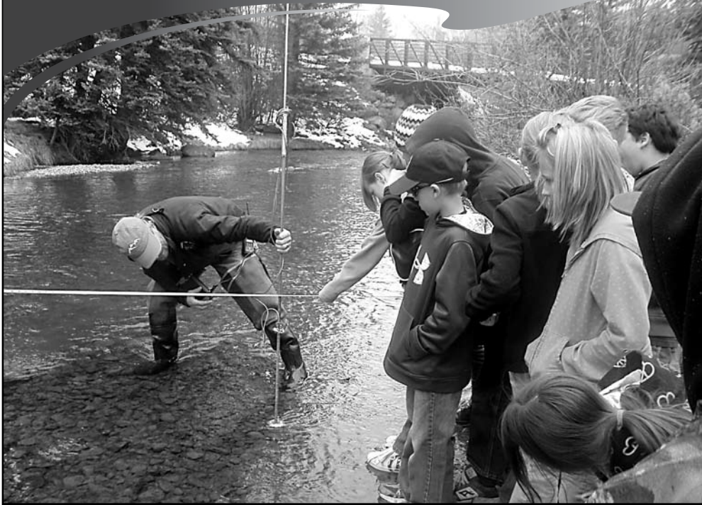
Mountain Village Water Department employee Patrick Drew shows 4th-grade students from Nucla and Naturita how to measure a streamflow with a bucketwheel meter on the San Miguel this spring.
