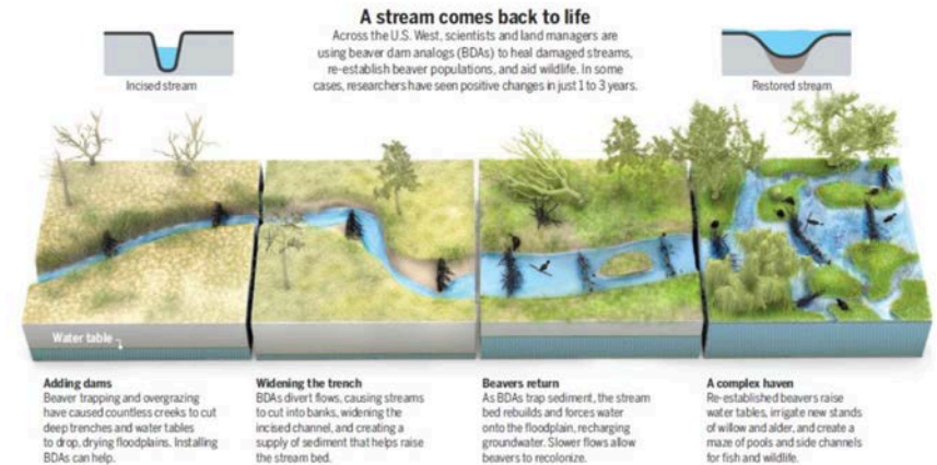
Figure 2. An example of beaver dam analogues (BDAs) mimicking beaver dam activity, and then the maintenance and expansion of beaver dam activity is taken over by actual beaver, and then they maintain a complex system state (Wheaton et al. 2019).
